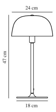
Voltage (V): 230 Volt IP degree: IP20 Maximum bulb wattage (W): 40 Class (Class 1, Class 2, Class 3): Class 2 (Double isolated) Socket type: E14 Switch placement: On the cable
