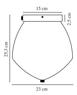
Voltage (V): 230 Volt IP degree: IP20 Maximum bulb wattage (W): 40 Class (Class 1, Class 2, Class 3): Class 2 (Double isolated) Socket type: E27
