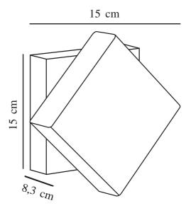
Voltage (V): 230 Volt IP degree: IP54 Class (Class 1, Class 2, Class 3): Class 1 (Earth contact) Socket type: LED - Nonreplaceable light source Dimmerable: True Parallel connection: True
