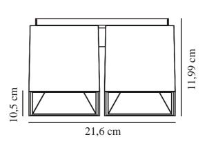
Voltage (V): 230 Volt IP degree: IP20 Maximum bulb wattage (W): 50 Class (Class 1, Class 2, Class 3): Class 2 (Double isolated) Socket type: GU10 Parallel connection: True
