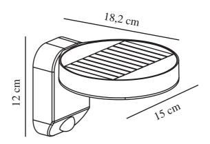
IP degree: IP44 Class (Class 1, Class 2, Class 3): Class 3 (12V)
