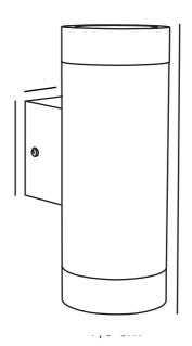
Voltage (V): 220-240 Volt IP degree: IP54 Maximum bulb wattage (W): 28 Class (Class 1, Class 2, Class 3): Class 1 (Earth contact) Socket type: GU10 Parallel connection: True
