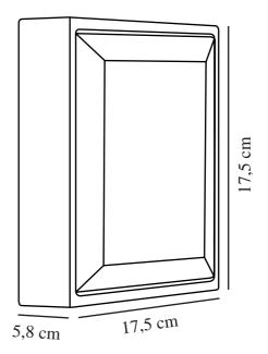
IP degree: IP54 Class (Class 1, Class 2, Class 3): Class 2 (Double isolated)
