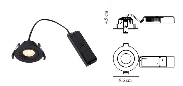
Voltage (V): 220-240 Volt IP degree: IP44 Class (Class 1, Class 2, Class 3): Class 2 (Double isolated) Socket type: LED – Non-
