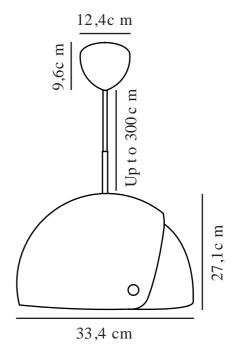
Voltage (V): 220-240 Volt IP degree: IP20 Maximum bulb wattage (W): 15 Class (Class 1, Class 2, Class 3): Class 2 (Double isolated) Socket type: E27 Parallel connection: False
