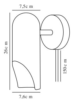
Voltage (V): 220-240 Volt IP degree: IP20 Maximum bulb wattage (W): 8 Class (Class 1, Class 2, Class 3): Class 2 (Double isolated) Socket type: GU10 Switch placement: On the wall
