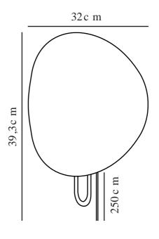
Voltage (V): 220-240 Volt IP degree: IP20 Maximum bulb wattage (W): 25 Class (Class 1, Class 2, Class 3): Class 2 (Double isolated) Socket type: E27 Switch placement: On the cable
