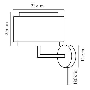
Voltage (V): 220-240 Volt IP degree: IP20
