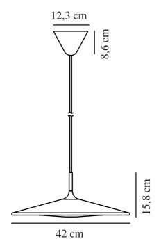
Voltage (V): 220-240 Volt IP degree: IP20 Class (Class 1, Class 2, Class 3): Class 2 (Double isolated) Socket type: LED – Nonreplaceable light source Dimmerable: True Parallel connection: False
