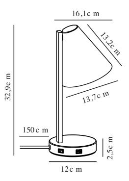
Voltage (V): 220-240 Volt IP degree: IP20 Maximum bulb wattage (W): 40 Class (Class 1, Class 2, Class 3): Class 2 (Double isolated) Socket type: E14 Switch placement: On the table/ground base Parallel connection: False
