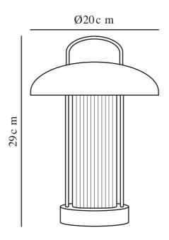
Voltage (V): 3,7 Volt IP degree: IP20 Class (Class 1, Class 2, Class 3): Class 3 (12V) Socket type: LED Module Switch placement: On the fixture Parallel connection: False
