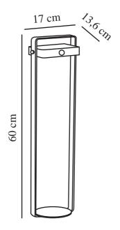
Voltage (V): 5 Volt IP degree: IP44 Class (Class 1, Class 2, Class 3): Class 3 (12V) Socket type: SolarLed Switch placement: On the fixture Parallel connection: False
