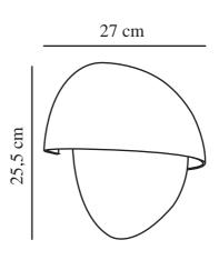
Voltage (V): 220-240 Volt IP degree: IP44 Maximum bulb wattage (W): 25 Class (Class 1, Class 2, Class 3): Class 2 (Double isolated) Socket type: E27 Parallel connection: True
