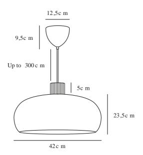
Voltage (V): 220-240 Volt IP degree: IP20 Maximum bulb wattage (W): 25 Class (Class 1, Class 2, Class 3): Class 2 (Double isolated) Socket type: E27 Parallel connection: False
