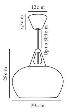
Voltage (V): 230 Volt IP degree: IP20 Maximum bulb wattage (W): 60W Class (Class 1, Class 2, Class 3): Class 2 (Double isolated) Socket type: E27 Dimmerable: Yes with compatible
