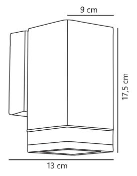
Voltage (V): 230 Volt IP degree: IP44 Maximum bulb wattage (W): 20 Class (Class 1, Class 2, Class 3): Class 1 (Earth contact) Socket type: GU10 Parallel connection: True
