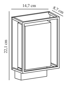
Voltage (V): 230 Volt IP degree: IP44 Class (Class 1, Class 2, Class 3): Class 1 (Earth contact) Socket type: LED – Nonreplaceable light source Parallel connection: True
