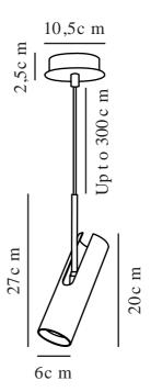
Voltage (V): 220-240 Volt IP degree: IP20 Maximum bulb wattage (W): 8 Class (Class 1, Class 2, Class 3): Class 2 (Double isolated) Socket type: GU10 Parallel connection: False
