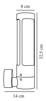
Voltage (V): 230 Volt IP degree: IP44 Maximum bulb wattage (W): 8 Class (Class 1, Class 2, Class 3): Class 1 (Earth contact) Socket type: GU10 Parallel connection: True
